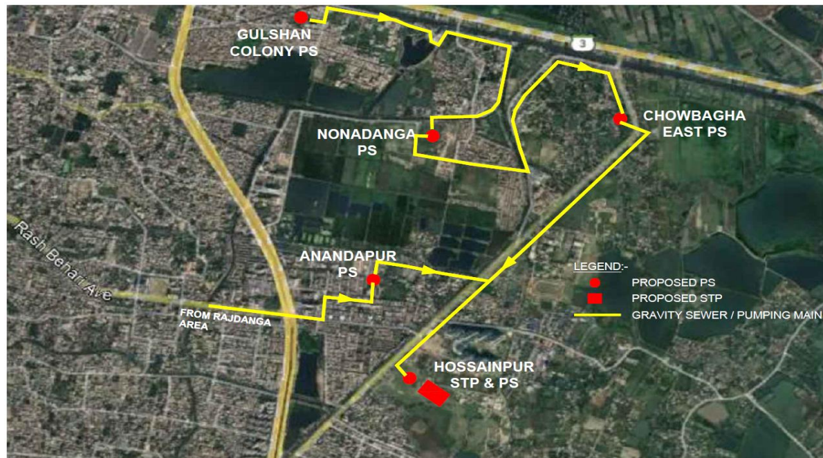
Figure 3: Transmission of DWF to proposed Hossainpur STP
